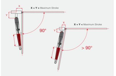
• If X+Y > Maximum Stroke, the opening angle of the gate will be less than 90°.
