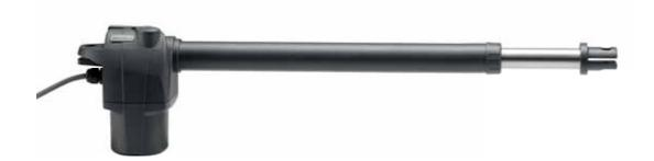
Irreversible electromechanical geared motor, available with power options 230 VAC or 24 VDC. Ideal for automation devices for wrought iron gates, this product is very small and suitable for a quick and easy installation. Worm screw protected by a scraper ring and stainless steel stem, suitable for dusty or sandy environments, or places with aggressive weather conditions. Available in right or left side versions.
