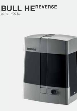
Reversible 230 Vac gear motor for sliding gates up to 1400 kg. Equipped with control unit with integrated receiver and encoder, ideal in condominiums for particularly intensive use. The electric brake guarantees the irreversibility of the actuator in the presence of a power supply.
