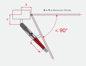
In standard applications, with inward opening, it is good practice to keep the dimensions X and Y almost equal to each other and restrict the difference between them to around 40 mm maximum to **avoid large changes in the speed of the gate during the maneuver:**
