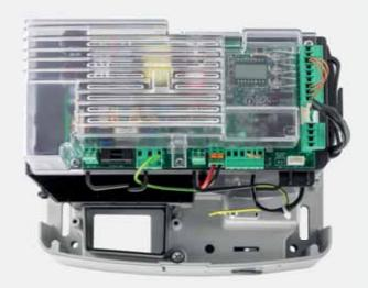
24 Vdc gear motor for sliding gates up to 1500 kg, ideal for intensive use. The built-in control unit, unique for all versions and accessible from above, makes it possible to memorize up to 2048 transmitters. The 115/230 Vac switching power supply reduces consumption (0.8 W) and secures a long lifespan of the actuator. Possibility of integration with KNX home automation systems through the specific X.BE card and remote programming thanks to the pro.UP interface card and the BeUP application.
